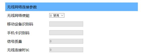
This feature is suitable for base stations that support 4G card insertion, with options for enabling and disabling, and displaying information related to IoT network cards
