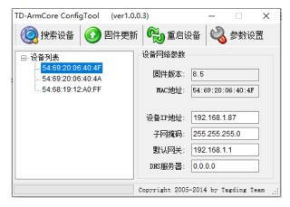
If the device IP address is changed to 192.168.1.87, click on parameter settings to complete the modification.
